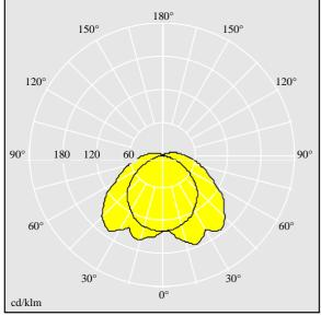
Colour Rendering Index min.: 80 Ballast: 1x HF ELXe Luminaire input power\*: 108 W Power factor = 0.95CELMA EEI: A2 Maintenance category: E - Dust-proof IP5X LOR: 0,58 ULOR: 0,04 DLOR: 0,54
