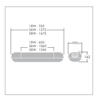
Lamp position: STD - standard Light Source: 2 x T26 / 58W Luminaire luminous flux\*: 6032 lmLamp luminous flux: 2 x 5200 lm Luminaire efficacy\*: 56 lm/W Lamp efficacy: 96 lm/W
