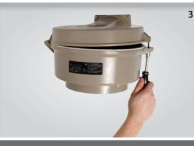
The main body can now be swung into place and secured using a screwdriver or nut driver. The terminal chamber is now sealed.
